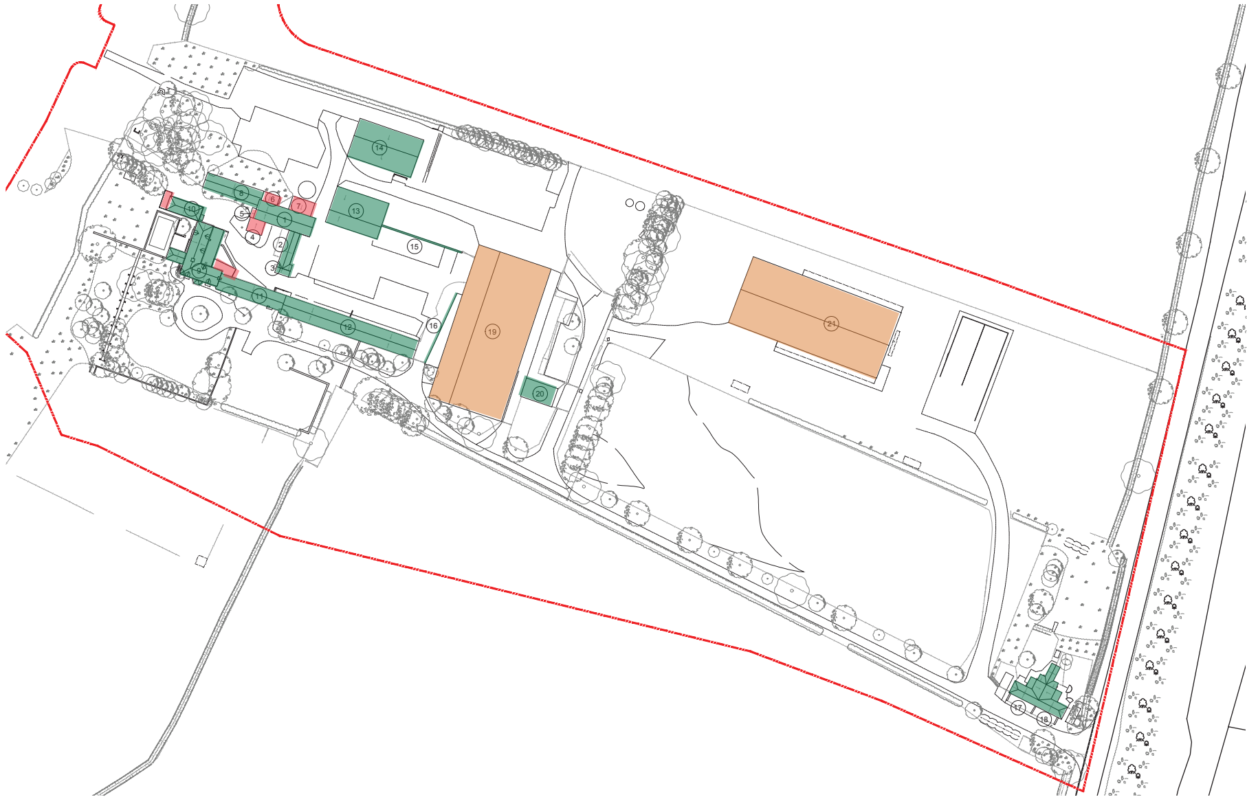
Fig 59. Site Plan, As Existing, with buildings to be restored in green, buildings which may have meantime uses in orange, and buildings to be removed in red.
